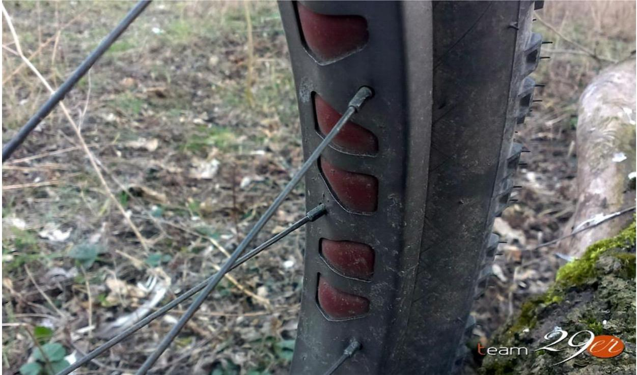
Heavily perforated rims are very difficult to convert to tubeless system, and so for the "ease" of life, Michael Travers offers a classic inner tube. But do not count on the low weight, because here we have two thick and heavy rubbers each weighing 400g! No pain, no gain!
