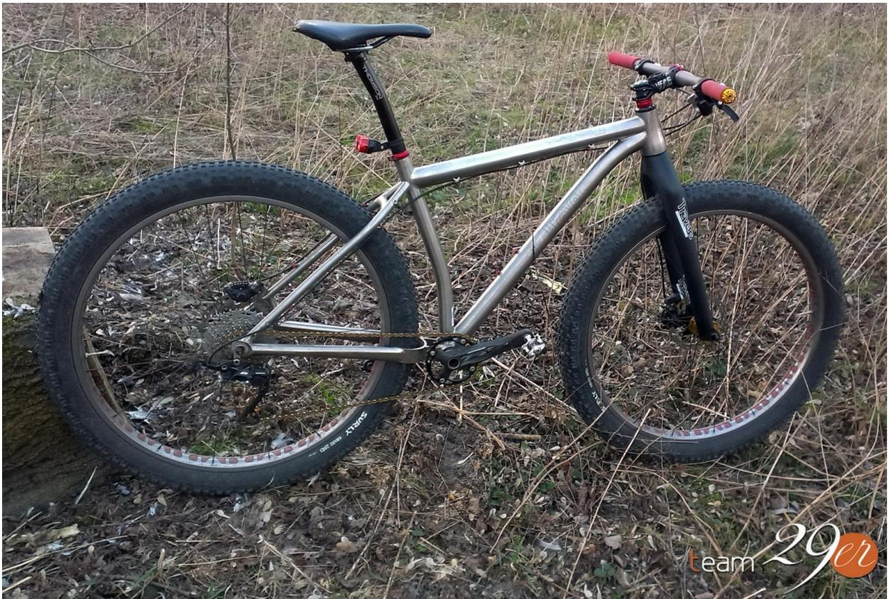
Michael Travers uses the popular and often used alloy Ti3Al-2.5V - the "equivalent" of AL7005. The main tube and the rear triangle have classical cross sections, maybe with the exception of slightly ovalized section of the down tube. Frame-builder did not make an effort to implement some technological and visual wonders. Simplicity, practical sense and minimalism - all are worth appreciating.
